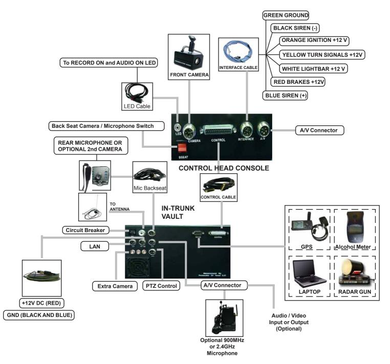
Figure 15: Description of Connections
