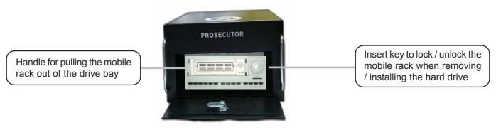
Figure 1: Removing Hard Disk
