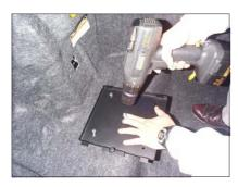
Place a hex head sheet metal screw at the middle hole of mounting plate.
