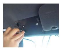
Attaching the control head mounting plate between the sun visors.
