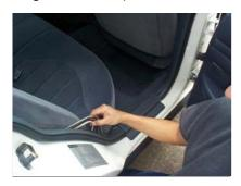
View of DB-25 and power cables coming from trunk, positioned behind the rear passenger side seat, heading toward front passenger seat. Note: cables go under carpet.
